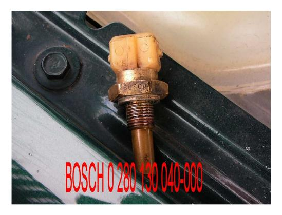
Use 19mm Wrench open & close ends to remove the sensor. I use the full size and a stubby (short) one to remove it. There will be some coolant will over flow but very minimal, so get the new one ready to install as soon as the old one is removed so you don't get too much coolant leaking out.
