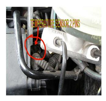
It's under the brake master cylinder and behind the camshaft. Just follow the black coolant metal pipe to the rear of the driver side camshaft.
