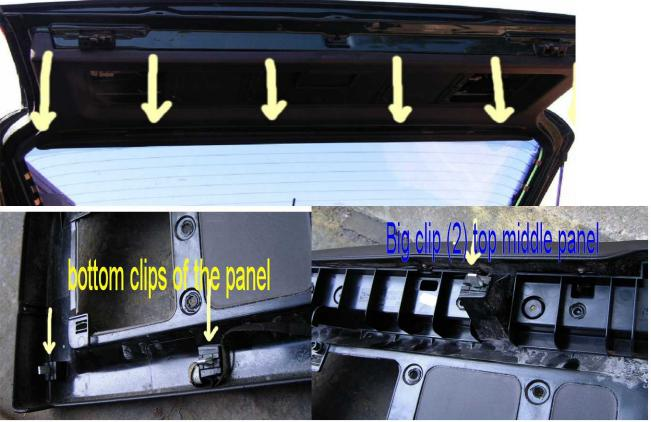
\*When removing middle clips, be careful not to break it. Use a long screw driver to pry up\*\*\*
