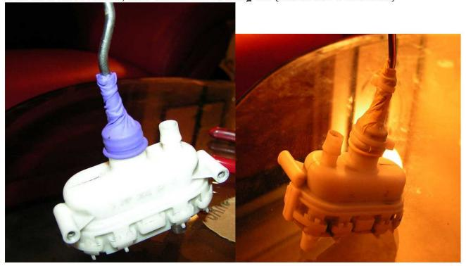
Tie wrapped both ends and wait for it to dry. I put some oil outside the final balloon because the balloon is very thin and sticky, when the pump actuated, it may get stuck. To be safe, I also pull another balloon over this one but not glue or tie wrap at all.
