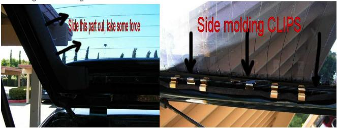
\*\*\*\*\* Pull these two sidemoldings out toward inside direction, wiggle and it does need some force.
