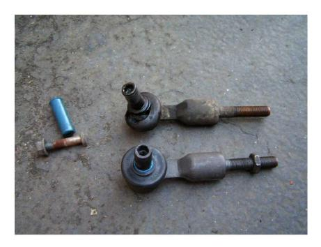
Put some lock-tight on the bolts 13mm & 16mm before putting it back in. Check the length on the new tie rod with the nut before screwing it back in.
