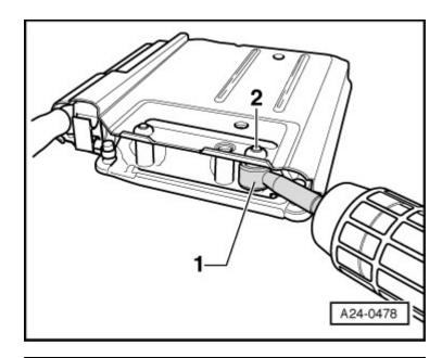
Grab bolt head -2- with locking pliers -1and turn shear bolt in direction of -arrow-.
