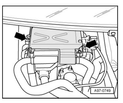
To increase difficulty with which ECM connectors can be accessed, ECM -1- is secured in a protective housing -5- with retaining tabs -2- and shear bolts -3 and 4-.
