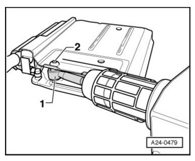
Then grab bolt head -2- with locking pliers 1- and turn shear bolt in direction of -arrow-
