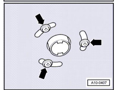
Remove bolts -arrows- for exhaust pipe of parking heater/auxiliary heater on noise insulation.
