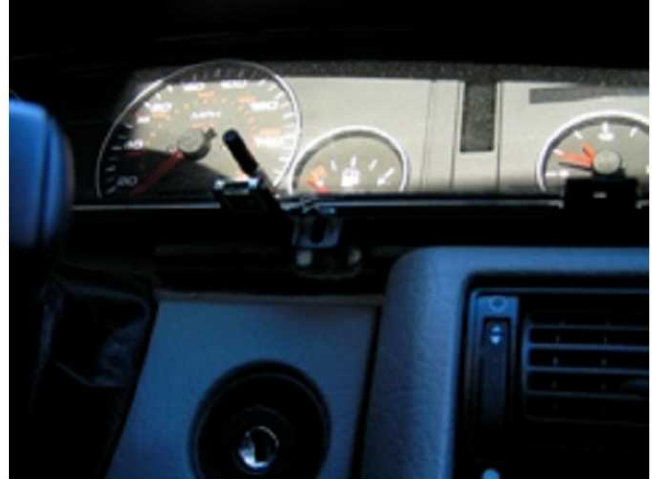
Pull out the instrument cluster bottom first.
