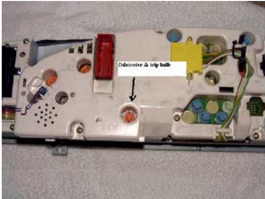
Odometer bulb Orange = 1.1W
