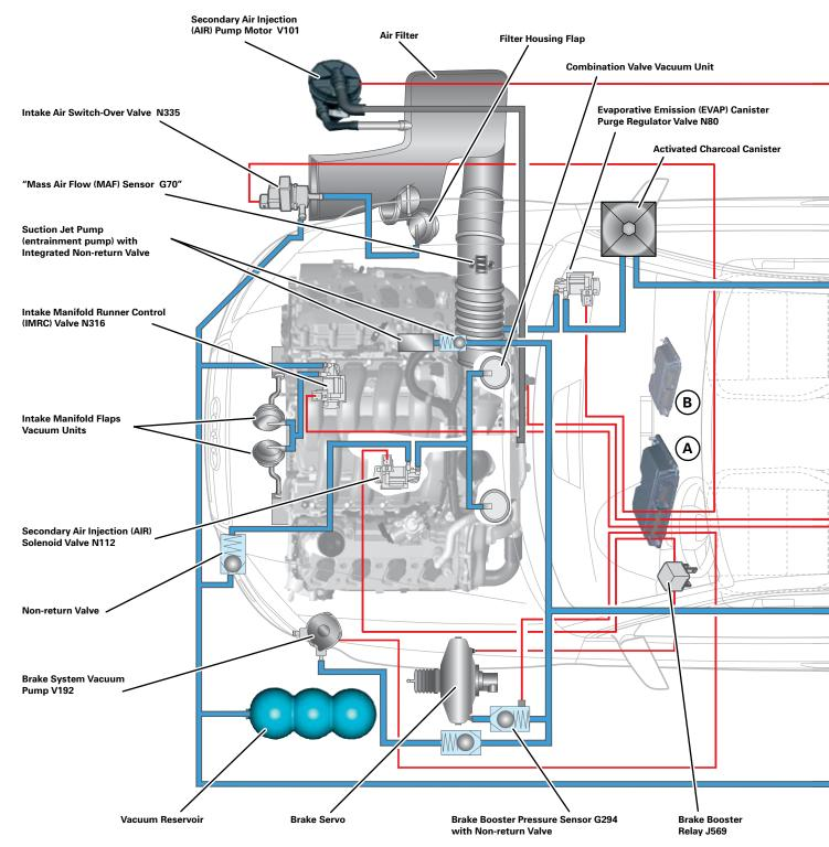
For this reason, in both engine versions, the required vacuum is produced by a suction jet pump and, if necessary, additionally by an electrical vacuum pump.
