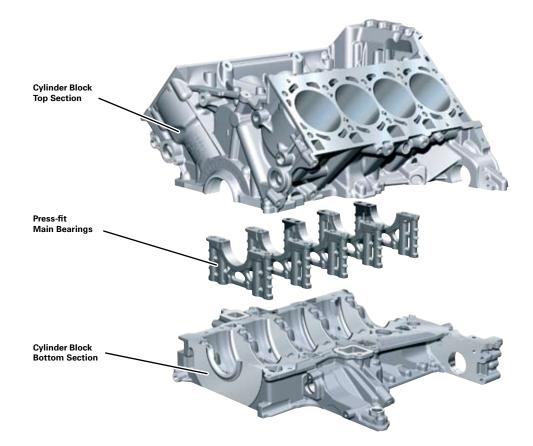
The cylinder crankcase lower section (bedplate bearing cross-member) is made of aluminum with press-fitted iron main bearing covers made of grade 50 nodular cast iron. It is centered using centering pins, sealed with liquid sealant and bolted to the cylinder crankcase.
