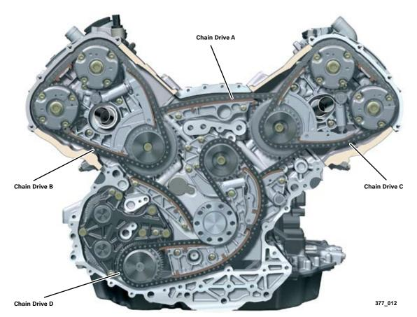
The timing gear concept is identical in all Audi V-engine series.
