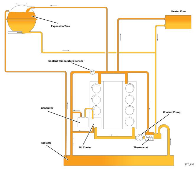
The cooling system in the new V8 engines was configured as a longitudinal-flow cooling system. The cooling water flows in on the outlet side and through the cylinder head gasket into the cylinder head, where it flows out longitudinally through the chain housing cover.
